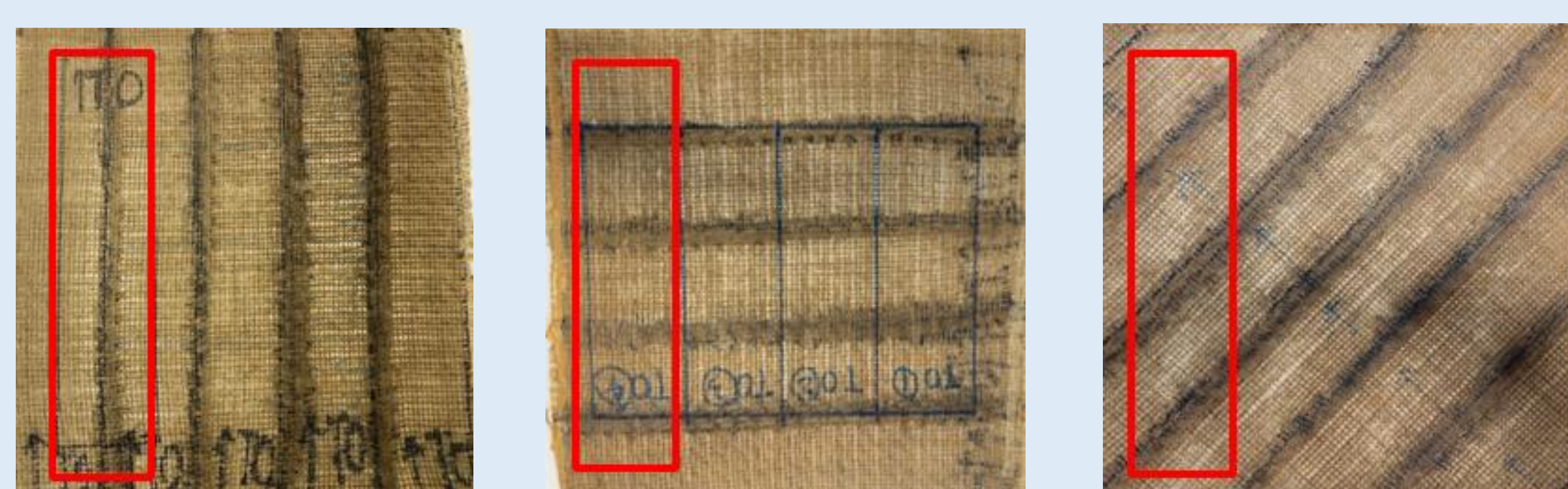
Figure 4. The different cutting directions for specimens
